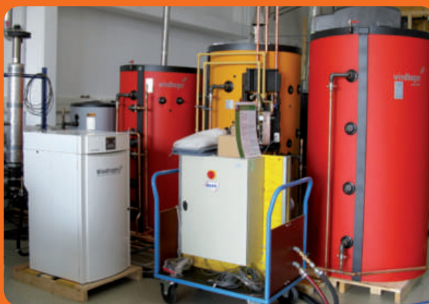
Figure 21: small-scale hybrid system composed of biomass boiler, solar thermal collector and sensible thermal energy storage (credits: Walter Haslinger, Bioenergy2020)
