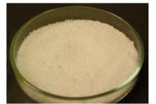
Figure 27: Sample of magnesium sulphate powder - one of the thermochemical materials under investigation. (Source: ECN, The Netherlands)
