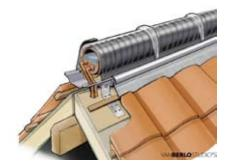
Figure 28: Example: A solar thermal roof-ridge collector is a "hidden" installation, which is already used in a few EU countries. It provides solar heat and also acts as a "standard" roof ridge. It has been developed primarily as an architectural solution to the integration of solar active roof elements, which will not impede subsequent roof alterations, such as the installation of a dormer window. (Source: Inventum, The Netherlands)
