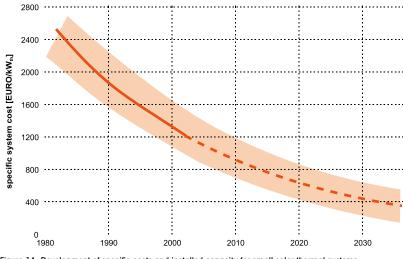
Figure 14: Development of specific costs and installed capacity for small solar thermal systems (forced circulation) in central Europe. (Source: ITW, University Stuttgart)
