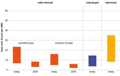
Figure 13: Typical cost ranges of domestic water/space heating with solar thermal, gas and electricity. (Source: ESTIF, 2008)
