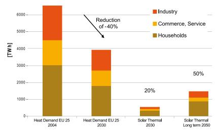
Figure 2: Contribution of solar thermal to EU heat demand by sector, assuming that the total heat demand can be reduced by energy conservation and a 40% increase in efficiency by 2030. (Source: AEE INTEC, 2008)
