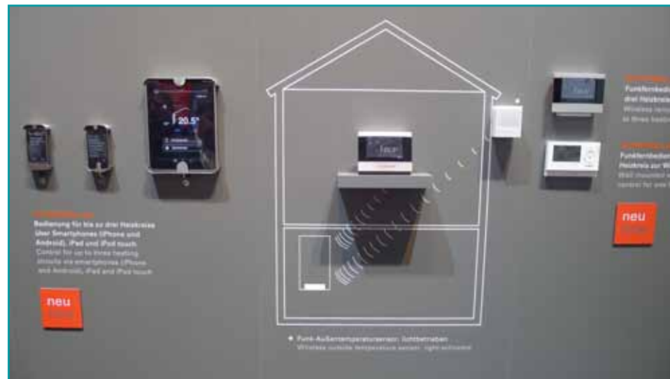
Figure 42 - ICT for remote control of the heating and cooling system (© Thomas Nowak, EHPA)
